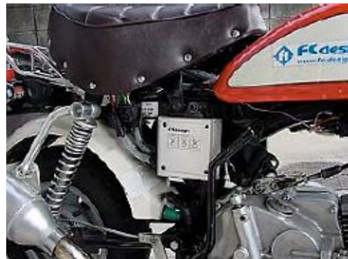
The harness kit is designed so that ECU is installed at the center of the vehicle.
