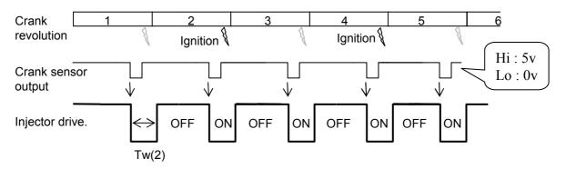
Tw(2) = [The injection time width value (WOT or ID)] / 2 + [the injector raction time]
