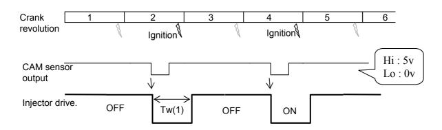
Tw(1) = [The injection time width value(WOT or ID)] + [The injector reaction time] The timing of starting injection is after the intake valve close in this figure.
