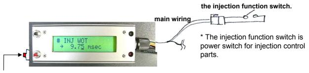
Meter function power switch (left side)
