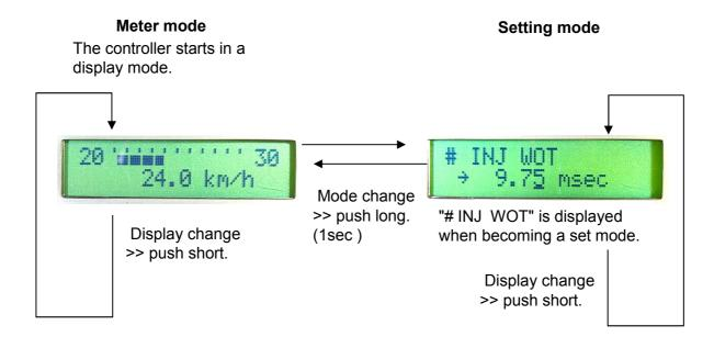
\* When the controller is turned on next time, it becomes a screen that had been selected at the end when it is turned off. (Last "Meter Mode" display.)
