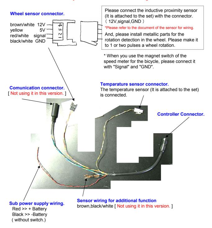
\* The controller doesn't using wheel sensor and temperature sensor to control the fuel injection.
