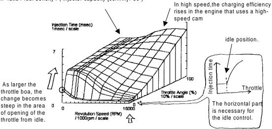
When becoming over 16000 rpm, ECU controls a Injection time by the parameter of 16000 rpm.
